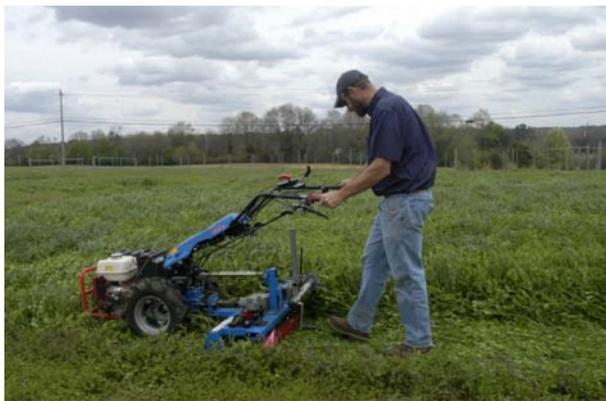
*Corey Kichler demonstrates an experimental attachment out of ARS helps roll and crimp cover crops for small no-till systems.*
