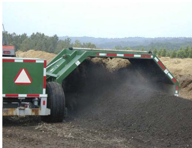
Windrow composting with specialized equipment that regularly mixes the compost. Photo by George Boyhan.
